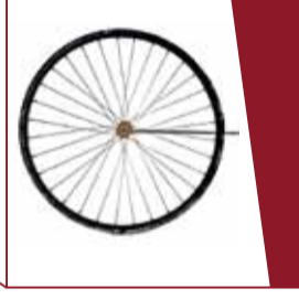
Bicycle tyre made of wire Rubber was scarce. Here is it substituted by a spiral wire.
